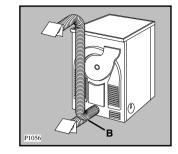
Once connected to the dryer, run the vent hose to the desired outlet point, ensuring that the run's overall length is less than 2 m, and that it contains no more than two bends. As to the outlet itself, if you have decided on a fixed wall/window grille, a good local builder's merchant should be able to supply you with the necessary fittings and installation advice.
